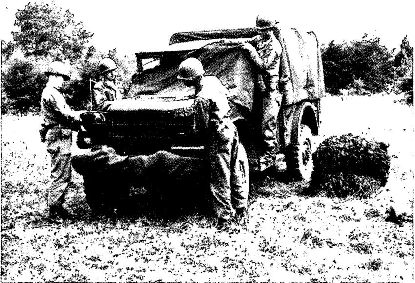
Figure 215. Crew covering windshield, lights, and reflectors.
